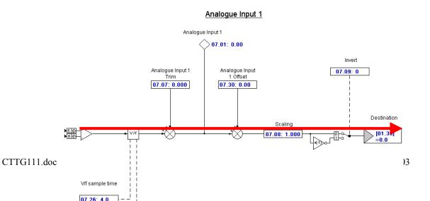
Once the signal has been confirmed at the terminal you should look at #7.01 to see if it changes with the change in reference at terminal5. #7.01 goes from +/-0%-100%. If it looks good check the destination of the speed reference at #7.10. Follow it to the destination and confirm the speed reference value is getting there and then through to #3.01.
